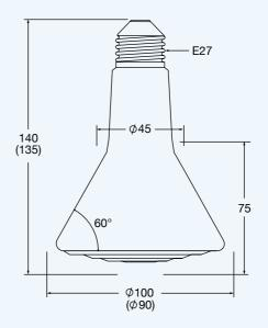
Figure: 51 Mounting dimensions and radiator dimensions ( ) in mm
